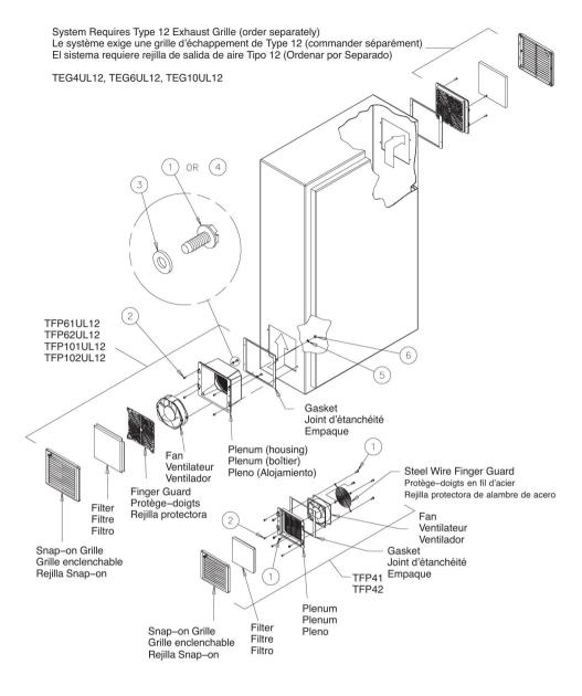
NOTE: To maintain UL type 12 rating, the airflow must be in the direction shown.
