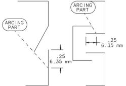
A barrier shall be secured in place by mechanical means such as mechanical fasteners.
